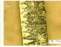
Scribed surface for 300 μm GaAs
